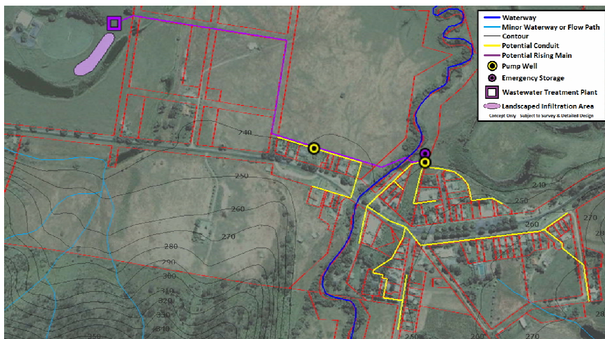
Figure 6.3: Schematic of wastewater strategy for Eskdale
