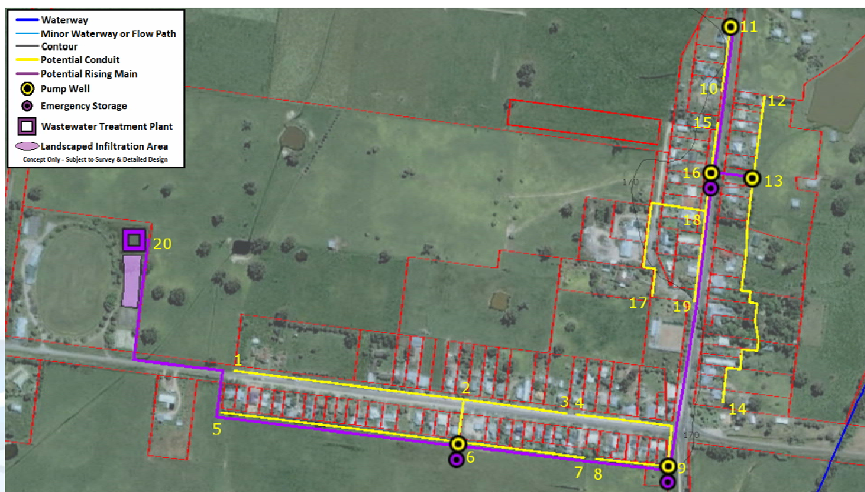
Figure 6.6: Schematic of wastewater strategy for Moyhu
