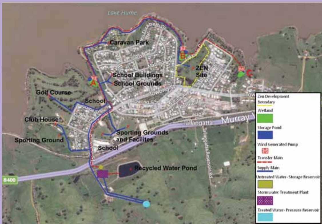
Figure 7: Diagram of the proposed stormwater harvesting and wastewater reuse strategy
